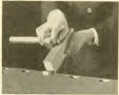
Fig. 5. The Marking Gauge in Use.
